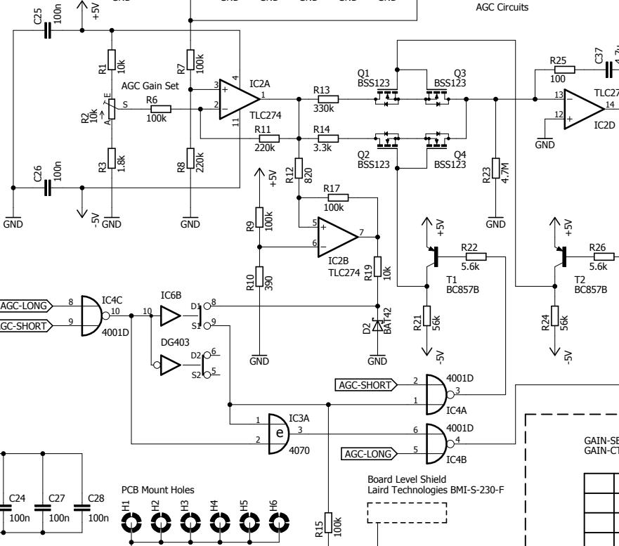
GAIN-SET Voltage Range: 0V (max gain) to 3V (min gain)
